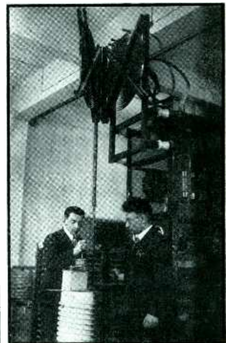
Fig. 6.—The authors with a high frequency vacuum tube generator with power output 20 kw used for hardening of steel parts
